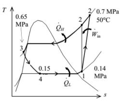
Then the rate of heat removal from the refrigerated space and the power input to the compressor are determined from
