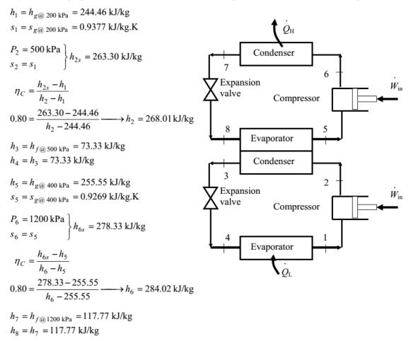
The mass flow rate of the refrigerant through the upper cycle is determined from an energy balance on the heat exchanger
